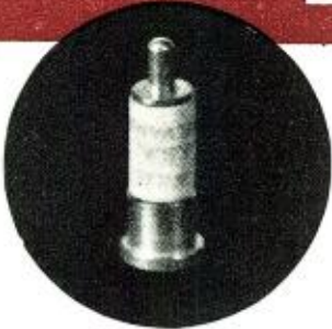
Fig. 2. Special u.h.f. fixed crystal detector employed in microwave frequency meters.
