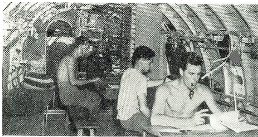
Interior of message-center plane, employed by the Signal Corps airborne radioteletype system in Japan. Left to right: radio operator, teletypist, and clerk.
