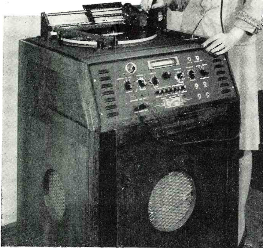
The completed sound reproducer. In this installation a recording unit complete with its amplifier is mounted on top of the cabinet as a single unit.
